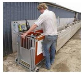
Whilst other weighing systems use the weigh head as the unit to capture, display and download weight data to a PC, the Handheld Stock Recorder is far more versatile as it will capture and record all of the information required for management of stock including the weights. It also allows the user to look up information on animals and record comments against them. 8 week weights, 20 week weights and wean weights can also be recorded.
